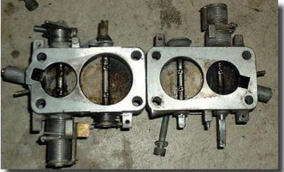
The intake manifold on an A1 is not machined to accept the larger throttle body, however, it can be ported to enable the use of the Audi throttle body. The alternative to porting it is to use a VW or Audi Fox or an Audi 4000 intake. There are bonuses to either apporach and both procedures are described below.
