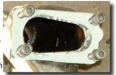
area can be opened up without worrying about breaking through. During the grinding process, use the WD-40 or other lubricant to keep the carbide burr or file from "loading up". Spray liberally and stop frequently to keep the cutter lubricated. Take your time and you'll get good results. Shown below is what the intake should look like when you're done:
