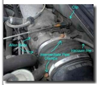
Remove your old throttle-body from the car. Do this by loosening the clamps holding the intermediate pipe to the throttle-body and pulling it off. Then remove any vacuum lines connected to the throttle body. There is probably only one in the back. Next, remove the clip holding the throttle cable on the linkage.
