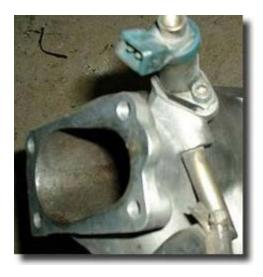
You can install the manifold with the valve in this location, but it will leave a good sized dent in your drip rail the first time the engine torques back. What's the solution? Note that the end on the fox intake is nice and flat...
