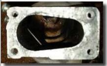
Now comes the fun part. You will have to port the intake manifold to match the new throttle-body. First, stuff the manifold with rags or paper towels so no chips or shavings go down the intake tubes. The alternative is the remove the manifold from the engine, which makes this job quite a bit easier. Make sure you count how many rags go in, and remember to count them
