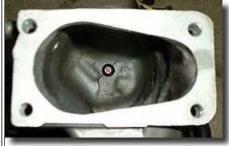
After you're done grinding out the intake manifold, use the shop-vac to clean out all the shavings and muck that you created. Make sure to get out as much as you can. Whatever you leave behind will undoubtably be sucked into the engine. Don't forget the rags too!! What was that count again?
