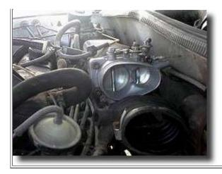
hook up all the lines again, you'll need to adjust the throttle cable. The Audi throttle-body's throttle linkage is further back so it puts tension on the cable, opening the throttle. If you don't loosen the cable a bit, you'll end up with a VERY high idle. Trust me, you don't want your car idling at 4,000 rpm. It's not really cool.
