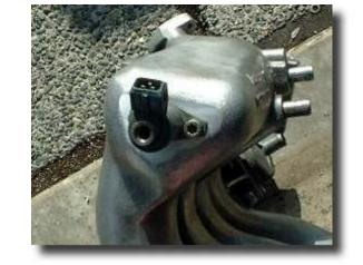
What about the old location for the cold start valve? Find a Digifant VW Fox and you will see it comes from the factory with a block off plate for the cold start valve. You can install that one, or make a plate of your own.
